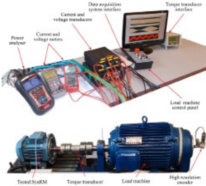
Fig. 5. Experimental setup and equipment for SynRM tests
